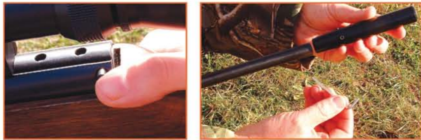
Above left: The auto-safety of the XS 20. Note, also, the scope arrestor holes.
