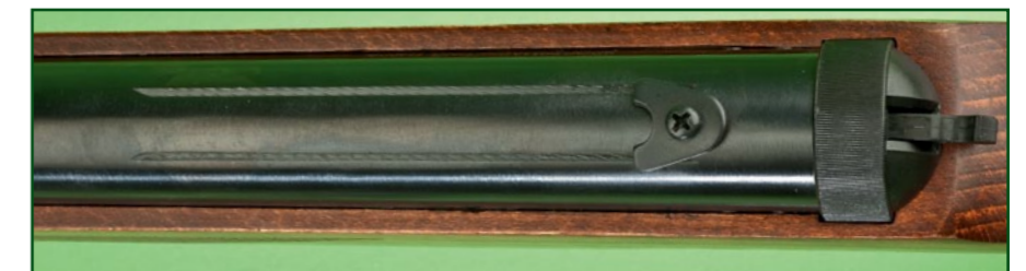
Above: The TH208's receiver is grooved for a telly and features an arrester plate at the end.
