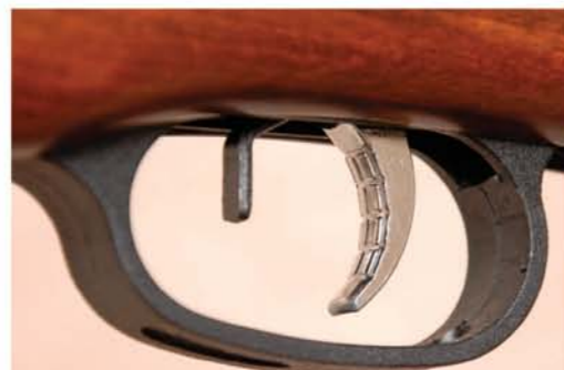
A broad trigger blade is a big help to accuracy
