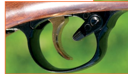
Below: The manual safety lever (on the other side of the guard), shown here in the 'on' position.
