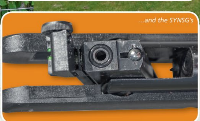
The SYN SG's plastic trigger blade is almost straight, and its pull-weight is lighter
