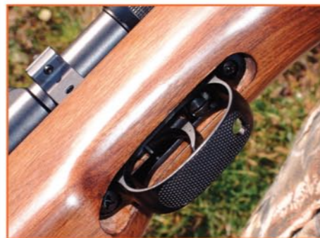
The trigger on the XS20 is not only two-stage, it's fully-adjustable, too!
