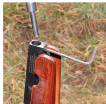
Just slide in the barrel of your choice, then re-tighten the grub screw
