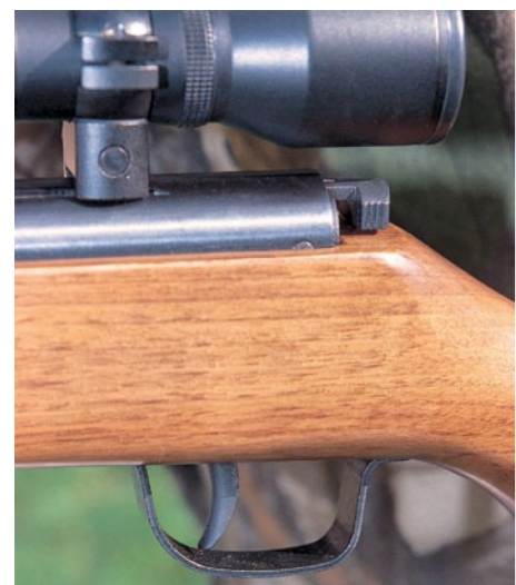
Details above show well engineered breech assembly and a familiar-looking safety set-up on the XS20. Below left, the XS15 exhibits more of the same - though I'd say that trigger could be further back within the guard which would help junior fingers to cope
