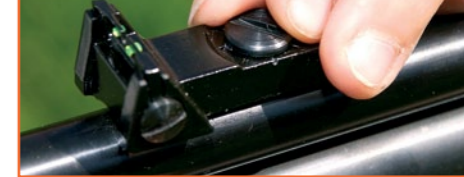
The fibre-optic rearsight is (finger!) adjustable.
