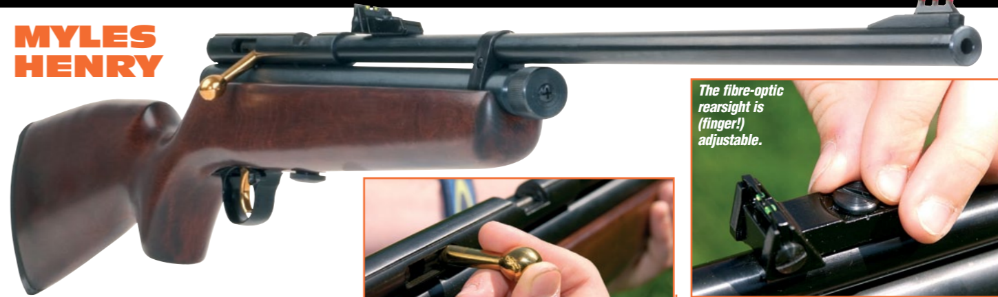
Above: Cocking the golden bolt. Right: The golden trigger blade. Note the 'F' and 'S' safety markings on the guard.
