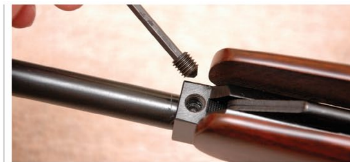
A large grub screw locks the barrel in place - just remove it to change calibres
