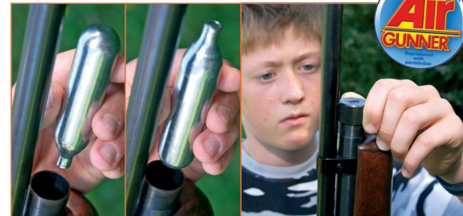
Below: The QB78 is powered by two, 12-gramme CO 2 capsules which you insert back to back (left and middle) before piercing with the screw-on cap (right).
