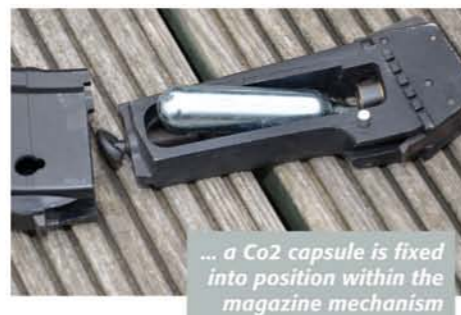
That small button releases the magazine internals...
