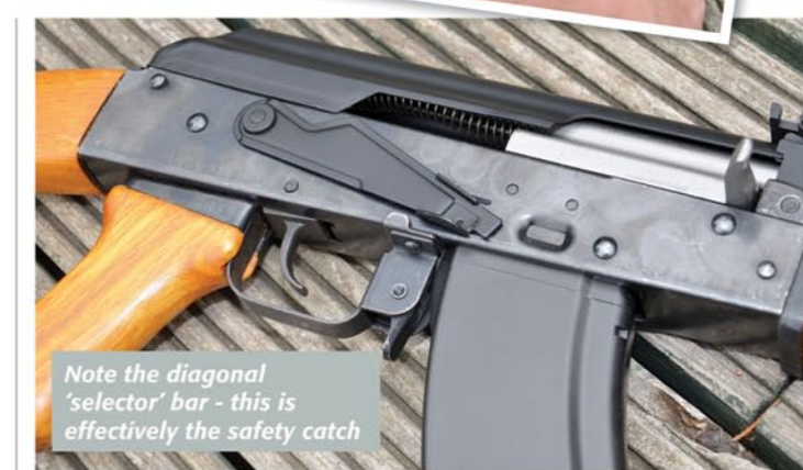
The small thumb catch allows the mag to be removed
