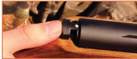
Above left: The auto-safety of the XS 20. Note, also, the scope arrestor holes.
