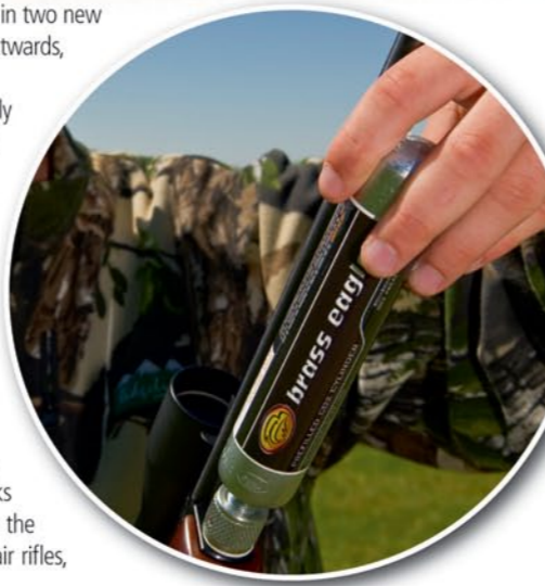
Top: Slot the two 12-gram capsules, facing outwards, into the TH78D's forend for power
